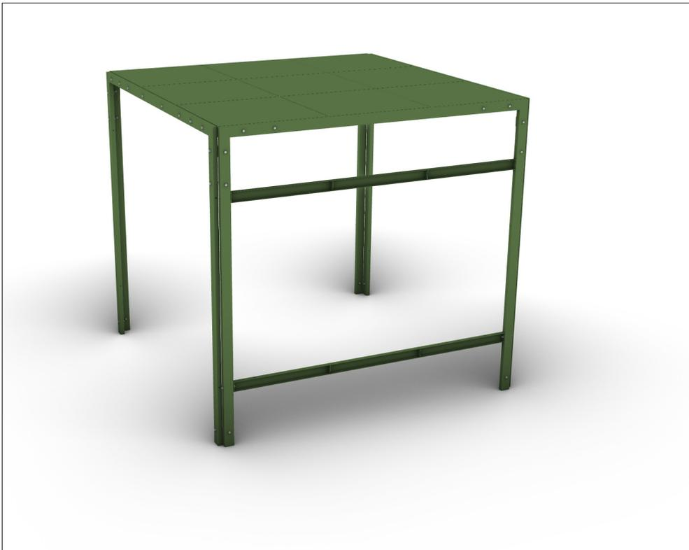
The position of the cross beams after attachment to the posts.
