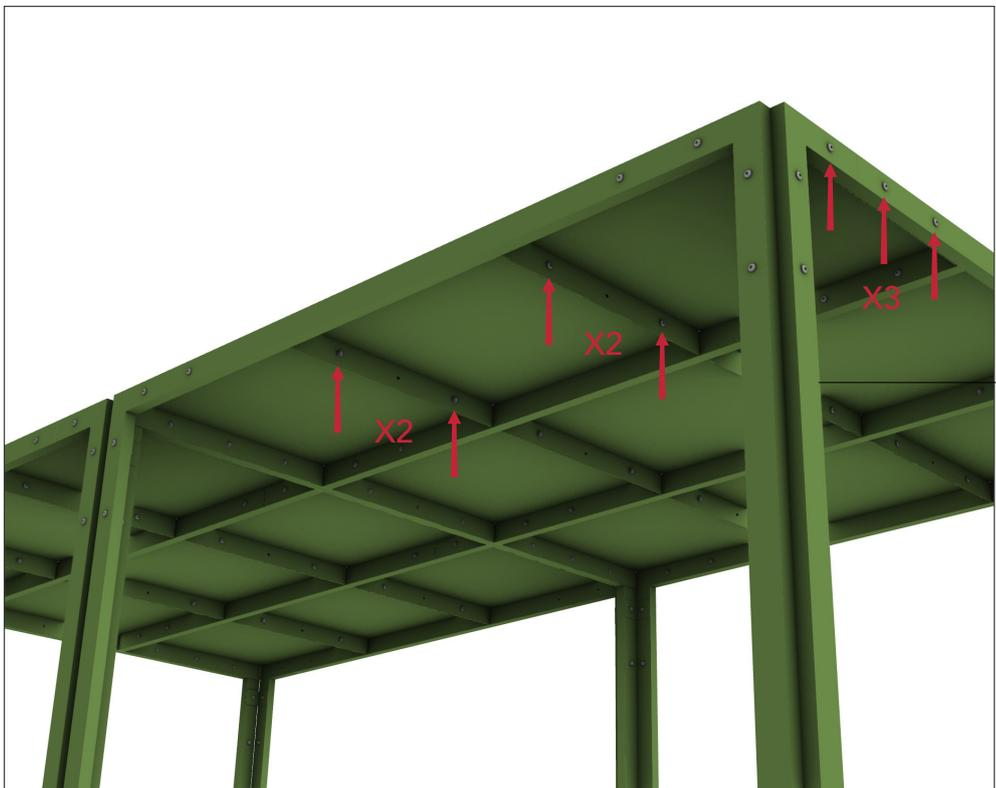
Each roof segment is attached with 2 bolts to the one next to it. 3 bolts when connected to the wall frames of the pergola.
