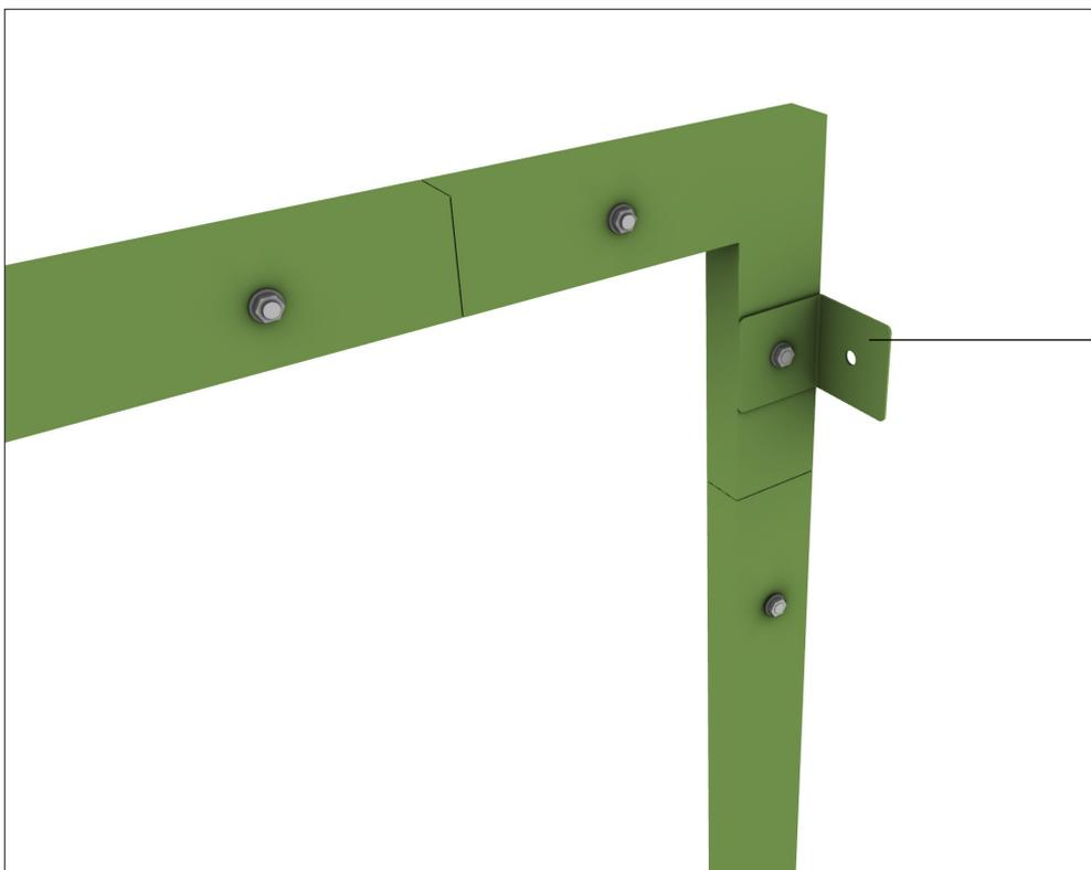
When attaching the leg posts of the 2 frames, connect also these L-shaped connectors as shown. 4 connectors that will hold the 4 sided structure together.
