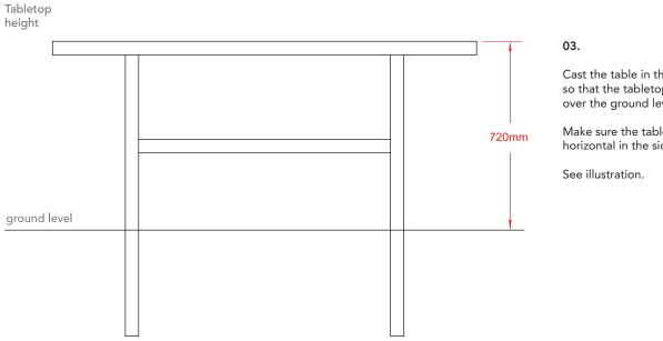
Cast the table in the chosen position, so that the tabletop height is 720mm over the ground level.
