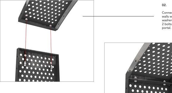
Connect the arch to the side walls with bolts, nuts and washers as seen in the images. 2 bolts on either side of the portal.
