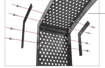
Connect the corner braces to the side frames with bolts, nuts and washers as seen in the images. 4 bolts on every support piece. In total 16 bolts.
