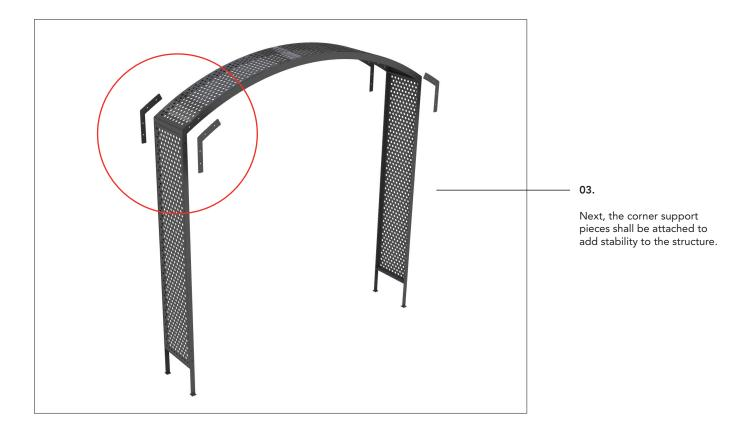
Connect the corner braces to the side frames with bolts, nuts and washers as seen in the images. 4 bolts on every support piece. In total 16 bolts.
