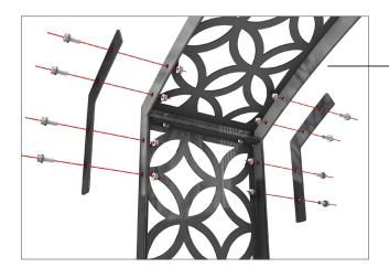
Connect the corner braces to the side frames with bolts, nuts and washers as seen in the images.
