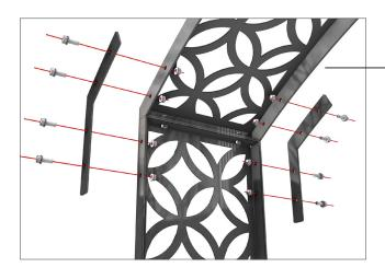
Connect the corner braces to the side frames with bolts, nuts and washers as seen in the images.
