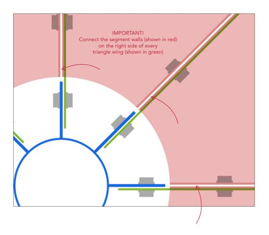
Connect the 8 canopy segments to the wings as shown here.
