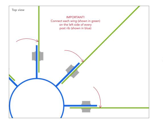
Connect the 8 triangle wings to the post as shown here.
