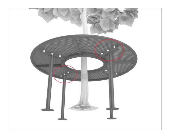
Connect the 2 seat halves and 2 leg structures using 6 nuts, bolts and washers.
